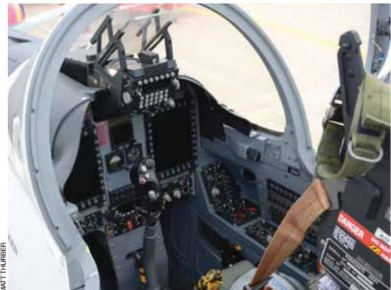
The cockpit of the Super Tucano includes dual six-by-eight-inch color LCDs for each pilot along with GPS navigation, night-vision-compatible lighting and autopilot.
